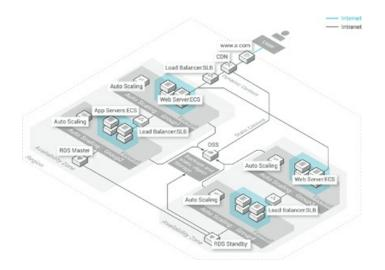
The architecture diagram shows how "Aliyun" cloud architect is powered by distributed servers and database services across multiple zones to ensure disaster recovery on deployment across multiple data centers, once the Server Load Balancer (SLB) detects the primary unavailable then it will direct all traffic to other in-service data centers.<sup>29</sup>
